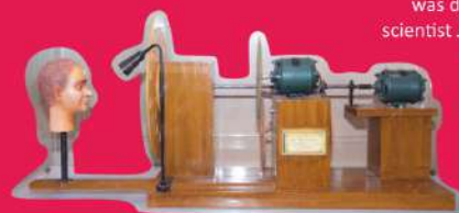
Baird Television - World's very first mechanical television set
